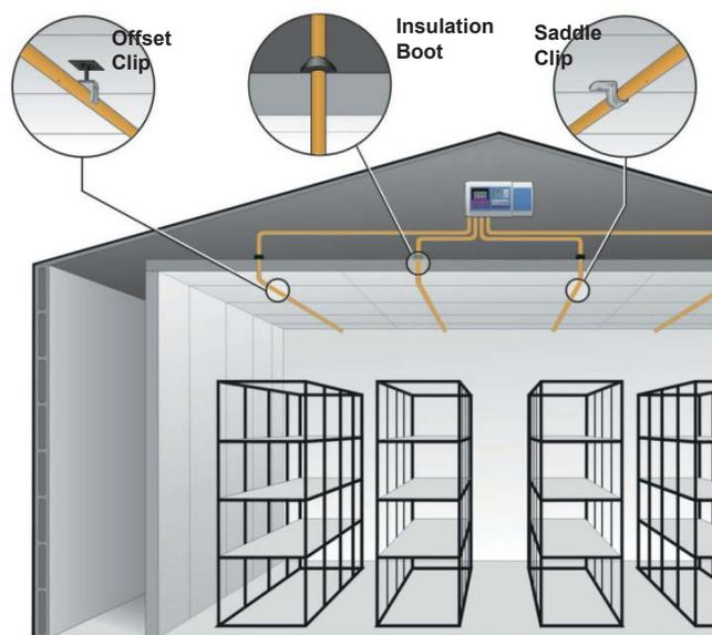
Figure 4. Cold Store Layout with Pipe Network
